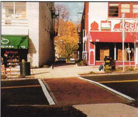
Figure 3.2.3.21: Crosswalks coordinated with alleys.
