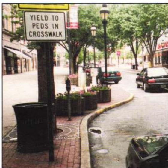
Figure 3.3.6.21: Curb extension and signage at mid-block crosswalk.
